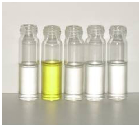
Figure 4. Colour changes of receptor ( R ) 2 in \text{CH}_3\text{CN} ( 5.0 \times 10^{-5} M) before and after the addition of 2 equiv of representative anions (from left to right: R , R + \text{F}^- , R + \text{Cl}^- , R + \text{Br}^- , R + \text{I}^- ).
